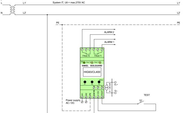
Three-phase IT system (3 x 440 VAC), HIG93/CL400 module with alarm signalling and with the remote test pushbutton
