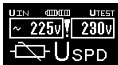
Fig. 3.4b Example of voltage measurement (USPD function)
