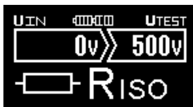
Fig. 3.5 Example of setting for insulation resistance measurement
