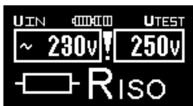
Fig. 3.4a Example of voltage measurement (RISO function)
