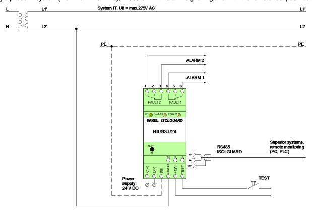
Three-phase IT system (3x500 V AC), HIG93T/24 with alarm signalling and with the remote test push-button
