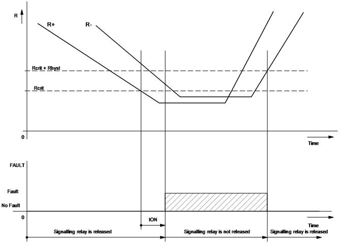
Picture 7: Insulation resistance fault evaluation
