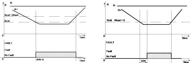
Picture 8: Insulation status fault evaluation with RtON or hysteresis zero value
