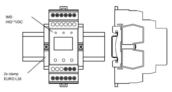
Picture 10: Device assembly in railway applications
