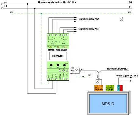
Picture 5: Recommended connection of device with MDS-D module
